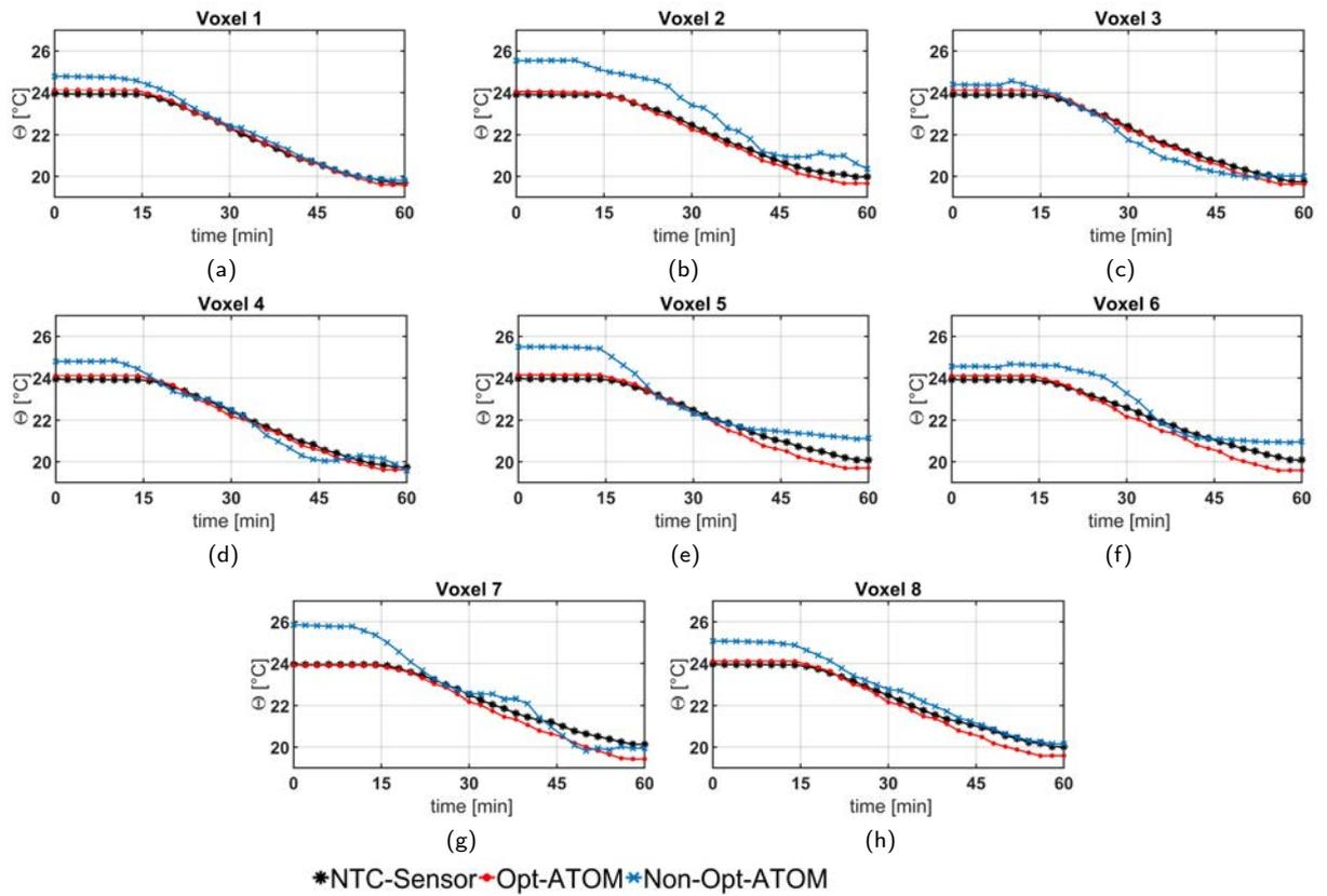
**Figure 7:** Measurement results during sessions 3 and 4 (Table 2), comparison of the temperatures of the NTC thermistors with ATOM temperatures for the both optimal and non-optimal cases within eight voxels separately.
