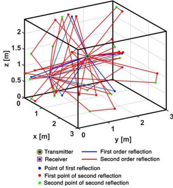
**Figure 1:** Three-dimensional representation of an image source model (ISM) with first and second order reflections.
