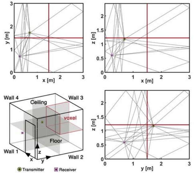
**Figure 4:** Subdivision of tomographic area. Each dimension of the room was divided in two parts evenly.
