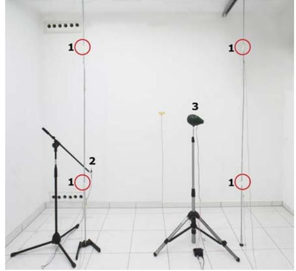
**Figure 2:** Experimental set-up in the climate chamber lab of the Bauhaus-University Weimar. 1) four of the eight mounted NTC thermistors which are superimposed, 2) receiver, and 3) transmitter
