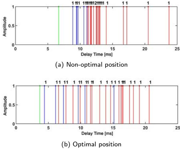
**Figure 3:** Comparing the reflectograms of (a) non-optimal and (b) optimal case. The number above the lines shows the number of sound paths arriving at that time within a threshold level of 0.1 ms. The order – green line: direct sound; blue lines: first order reflections; red lines: second order reflections – means how many times a sound signal is reflected at the room boundaries when traveling along the sound path from transmitter to receiver.
