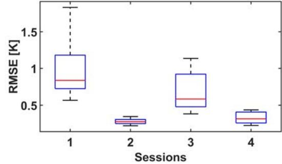
**Figure 9:** The root mean square error (RMSE) between the ATOM temperatures and NTC thermistors for each session, averaged over all voxels; black lines: maximum and minimum RMSE, red line: median RMSE, blue lines: 80%/20% quantile RMSE
