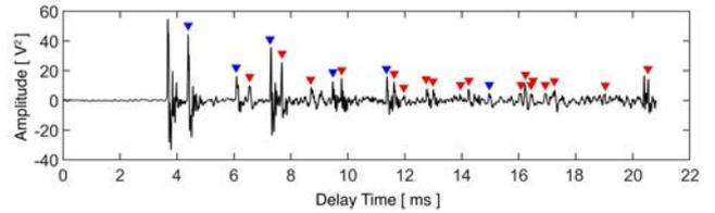
**Figure 5:** Calculated impulse response of the measured signal. The arrow signs above the reflections illustrate the selected travel-times, blue arrow signs are first order and red arrow signs are second order reflections.
