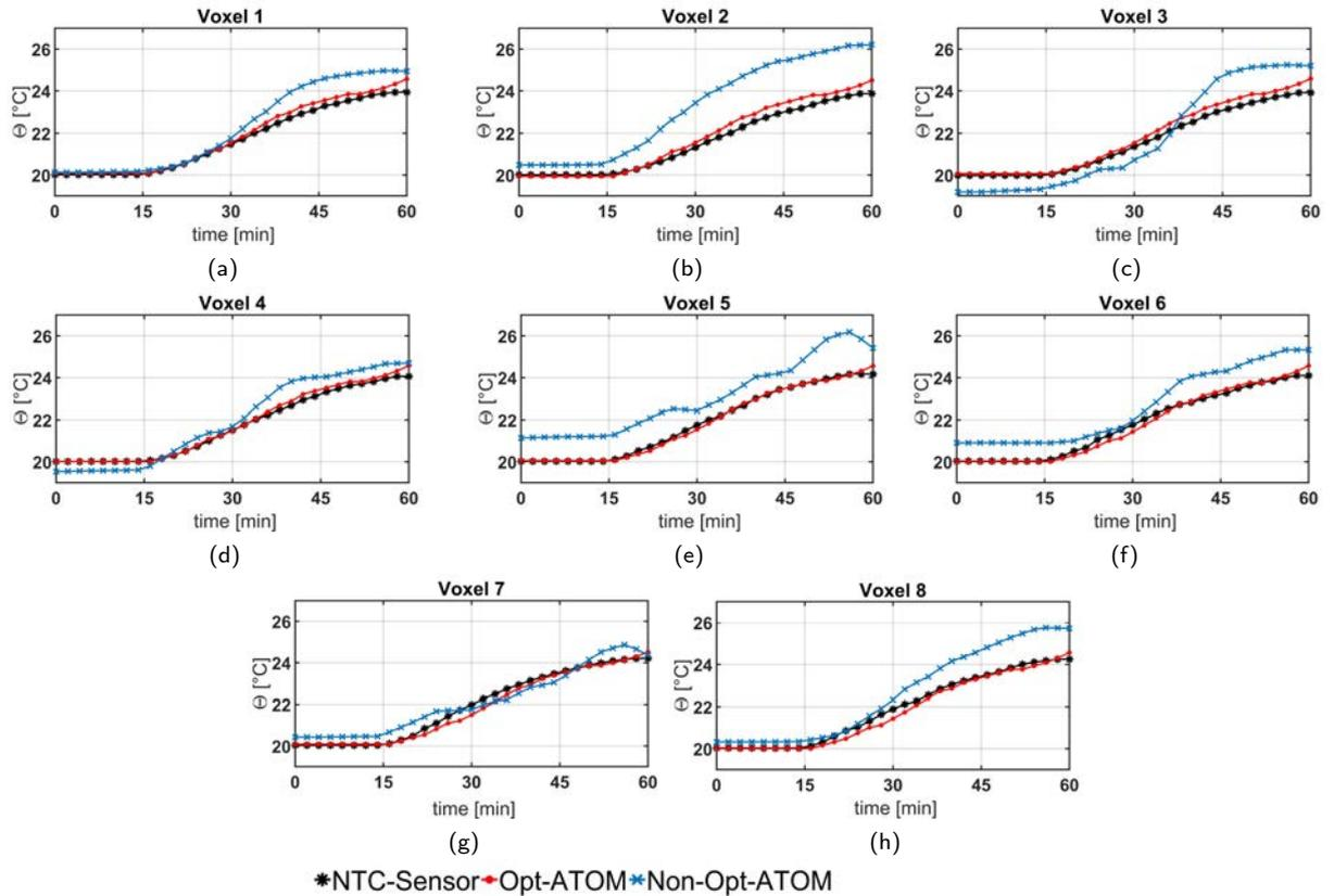
**Figure 6:** Measurement results during sessions 1 and 2 (Table 2), comparison of the temperatures of the NTC thermistors with ATOM temperatures for the both optimal and non-optimal cases within eight voxels separately.
