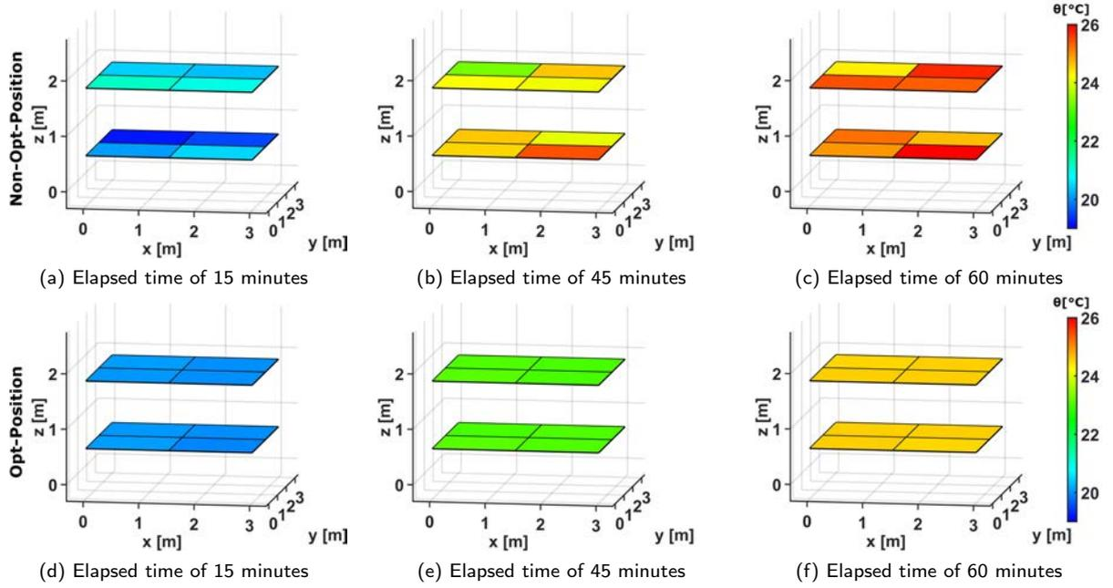
**Figure 8:** Three-dimensional representation of ATOM temperature distribution for the non-optimal (session 1) and optimal (session 2) positions. The color-bar of the optimal position illustrates the uniform variations of the temperatures inside the chamber in contrast to the non-optimal one.
