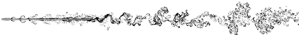
Fig. 9. Forced vibration simulations on a flat plate (aspect ratio B/D : 200): instantaneous vortex pattern.
