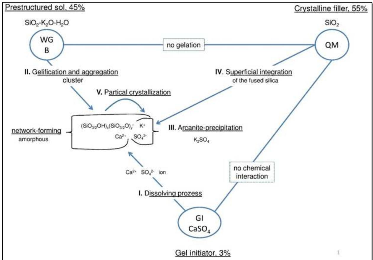
Figure 2: Components and their interactions with layer formation
