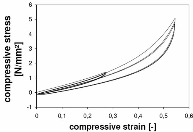
Figure 9: Elastomer behavior under cyclic loading [9]
