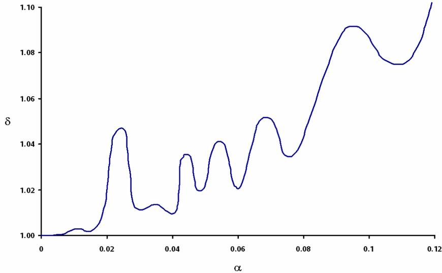
Figure 3: Effect of speed parameter ( $\alpha$ ) on the maximum dynamic deflection ( $\delta$ ) [5]
