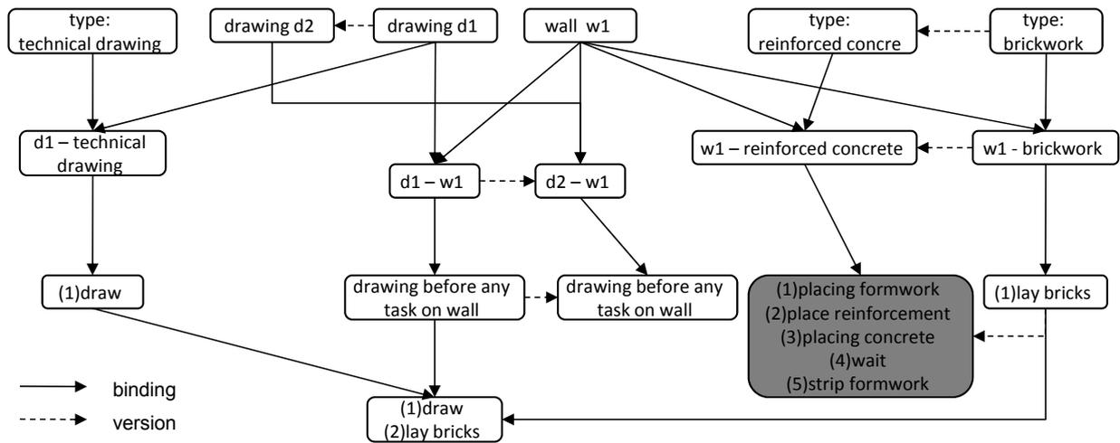
**Figure 12: Another sequence of task because reinforced concrete type**
