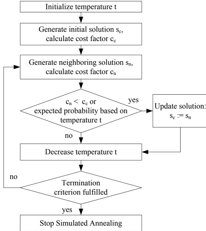
Figure 3: Simulated Annealing algorithm accordingly to [10]
