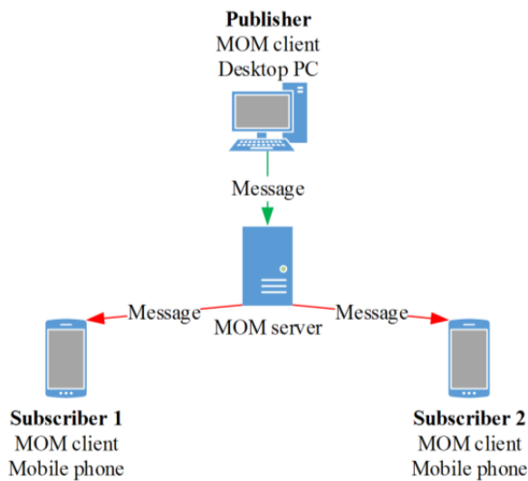
Figure 3: Publish/subscribe architecture with one publisher and two subscribers
