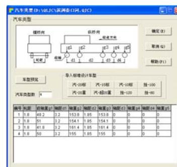
Fig.11 Interface of defining vehicle type
