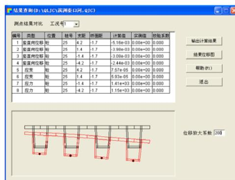
Fig.15 Interface of results display
