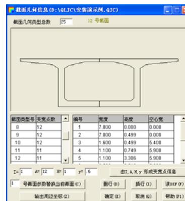
Fig.4 Interface of geometric dimension data of section
