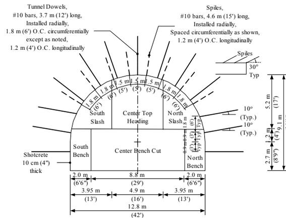
Tunnel Cross Section and Primary Support Type 3
