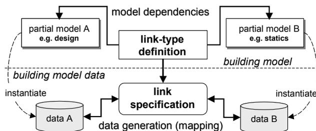
figure 5 : link-type definition and link specification
