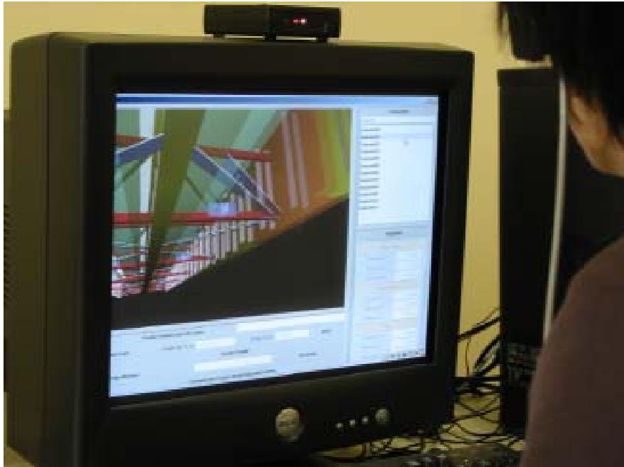
Fig. 6 A selected element of the design member is highlighted by changing its color from yellow to orange
