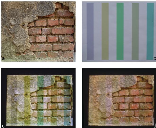
Fig. 7. Projection onto a striped wallpaper with saturated colors, without (c) and with (d) adaptive radiometric compensation.
