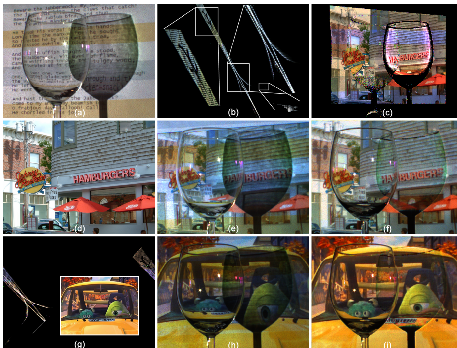
Fig. 3. A glass in front of a colored wallpaper (a). The acquired light transport matrix (b) is decomposed and used to compute a compensation image (c) for an input image (d). The result captured from the camera's point of view for the uncompensated (e) and the compensated (f) projection. Applying the inverse light transport matrix (g) allows a real-time compensation for displaying interactive content and movies - uncompensated (h) and compensated (i).
