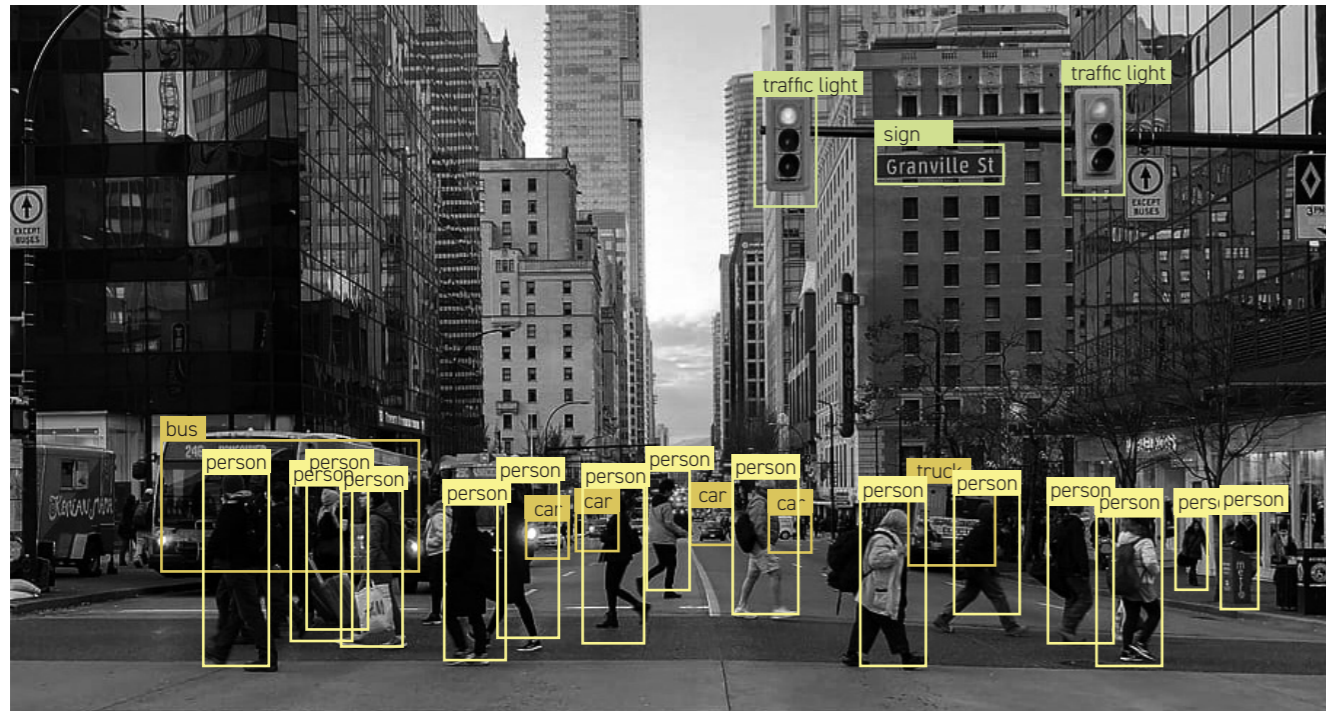
Figure 1.7: How a computer vision system uses object recognition to classify traffic lights, signs, persons, cars, trucks, busses
