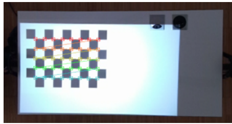
Fig. 42. Using a projected chessboard and OpenCV's cv::findChessboardCorners for projector calibration.
