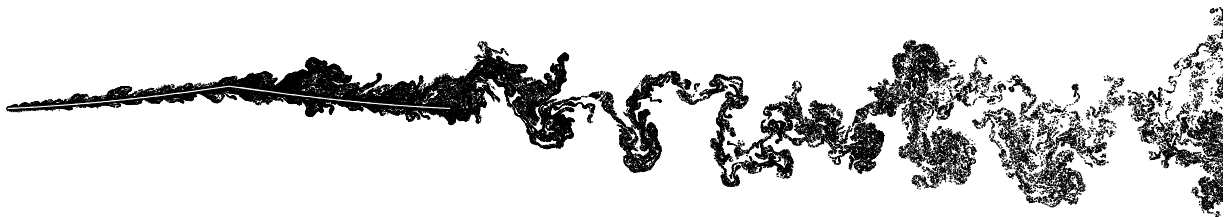
Figure 5.25: The convecting particles in free stream flow of 10 m/s around the membrane roof.
