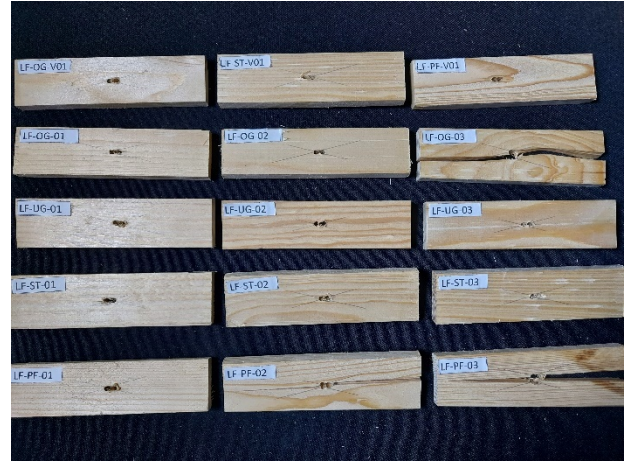
Figure 15: Embedment strength: specimens after the test
