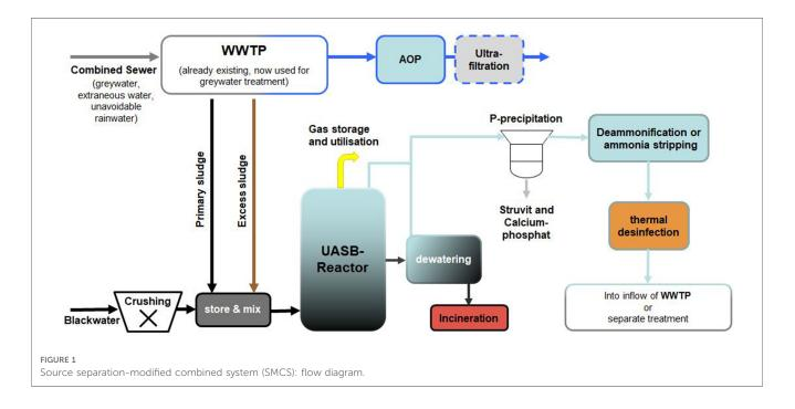
is passed once again through an Advanced Oxidation Process (AOP) stage and subjected to ultrafiltration, which further reduces AMR.
