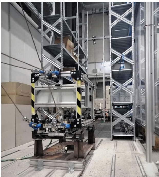
Fig. 4 A cable robot prototype as a storage and retrieval system at the University of Duisburg-Essen
