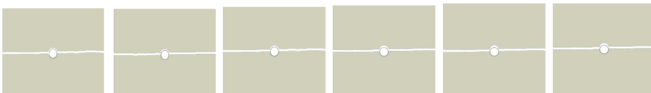
(a) (b) (c) (d) (e) (f) Figure 5.38: Crack pattern of \sigma^* 5% specimen (0.3 Mpa) with different G_f ratios. (a) G_f 100% (b) G_f 75% (c) G_f 50% (d) G_f 25% (e) G_f 10% (f) G_f 5%.
