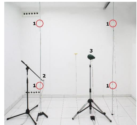
Figure 2. Experimental set-up in the climate chamber. 1) four of the eight mounted NTC thermistors, 2) receiver, and 3) transmitter
