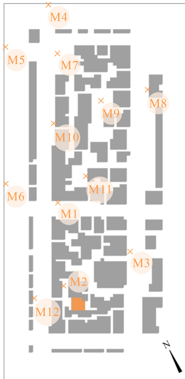
Fig. 10. The position of the probe points within the model. The marked building indicates the location where the indoor air temperature was probed
