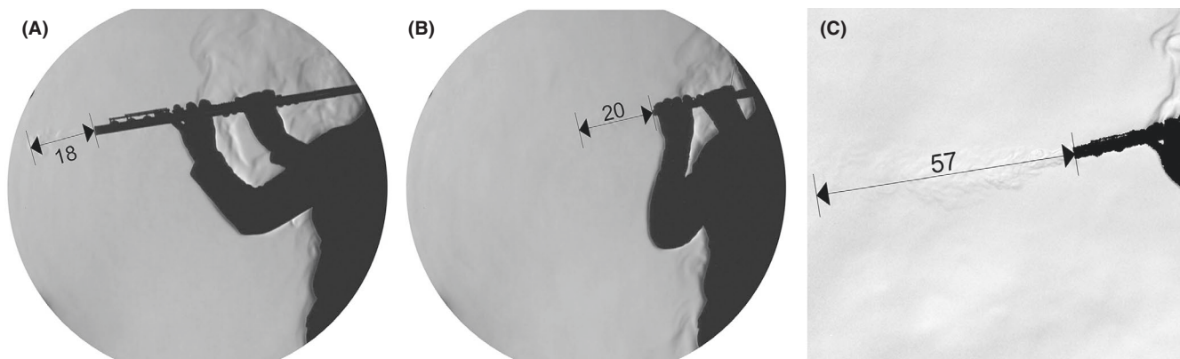
FIGURE 13 Maximal range of the air escaping from the foot joint of the grand flute while playing the note E4 \approx 330 Hz (A), of the piccolo while playing the note E5 \approx 659 Hz (B), and of the alto flute when playing the note G2 \approx 98 Hz (C) (cm)
