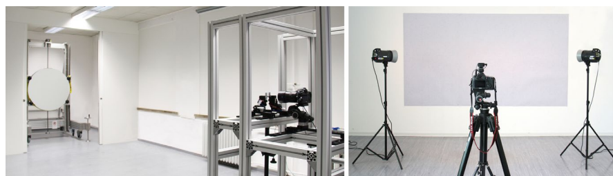
FIGURE 1 Setup of the single-mirror coincident schlieren system (left) and the BOS system (right) at the Department of Building Physics at the Bauhaus-University Weimar
