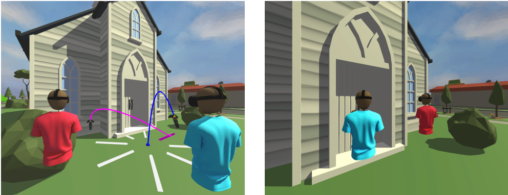
Figure 4.1: Our two-user jumping technique for remote collaboration allows the navigator (blue) to adjust the translational offset of the passenger (red) when planning a jump (left image). As a result, the group adjusts their formation during the jump, and the participants arrive at the appropriate locations to observe and discuss points of interest together (right image).
