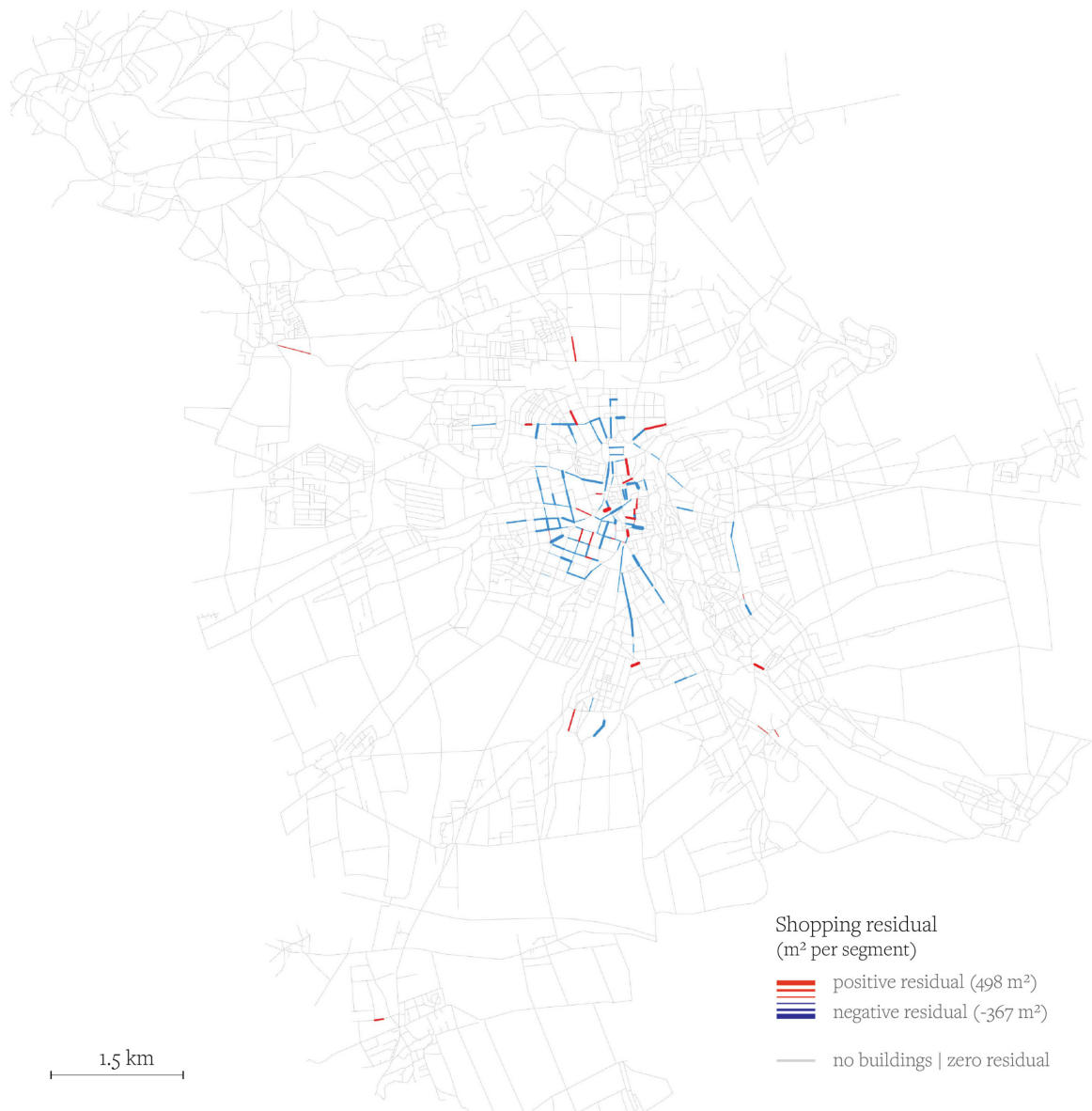
Figure 83. Residual map for predicted intensity of shopping activity. (Blue = negative residuals, Red = positive residuals, Black = prediction on target. The line thickness expresses the amplitude of the residual)
