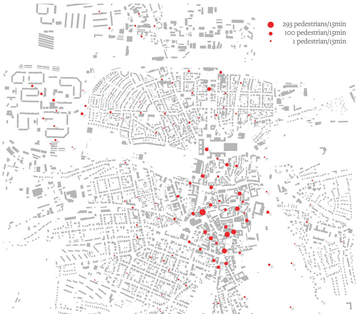
Figure 55. Distribution of empirical pedestrian counts (Pedestrian counting, 2016). The size of the circle represents the average number of passing-through pedestrians per 15-minute counting time.
