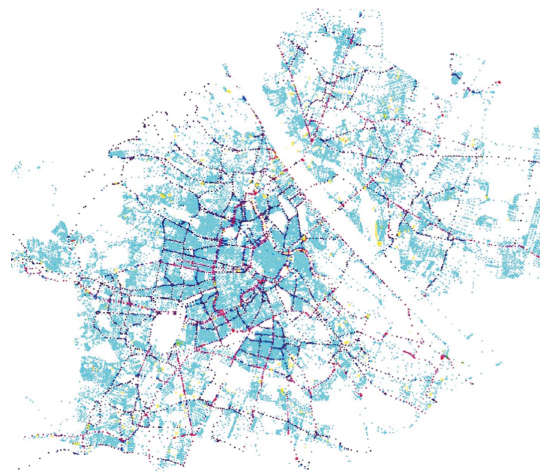
Fig. 15: Various road categories in Vienna. Colors represent a road category. Light blue represents residential roads, dark violet roads of highest hierarchy. For each type, individual properties such as avg. speed can be defined. Source: Author
