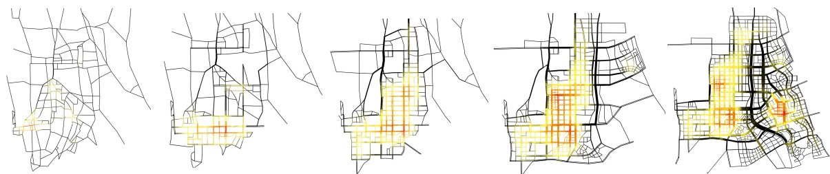
Fig. 60: Street network analysis for the Lanzhou New Area. From top to bottom: 2010; 2013; 2015; masterplan. Thickness of the line represents global betweenness centrality; Colors indicate local betweenness (radius = 1800m), red indicates high, black low, values. Source: Author
