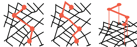
Fig. 28: Adding links to the network (2). Left: user input. Middle: background calculation: shortest path via road network from one station to the next Right: Visualization of graph structure with added bus line (in red: added nodes and edges). Source: Author
