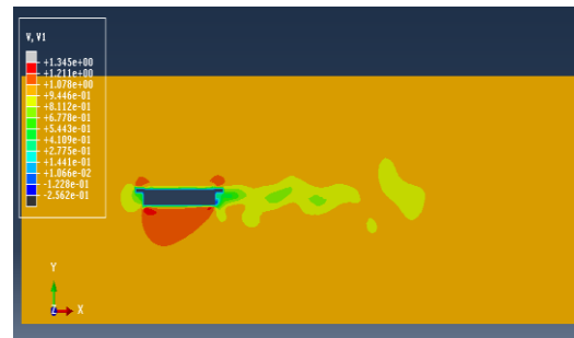
Figure 4.5 Vortex shedding two-way V=1 m/s
