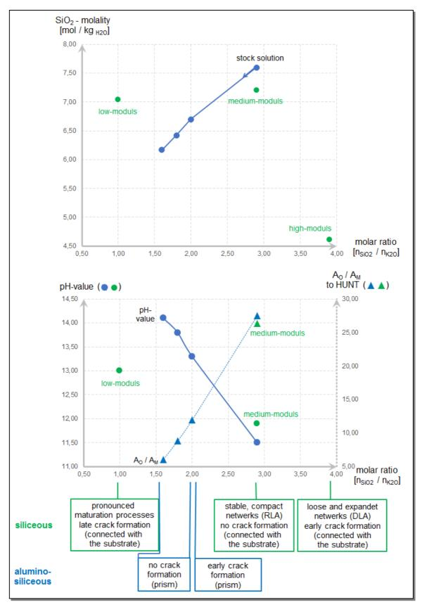
Figure 3: Potassium water glass solutions represented by the molar ratio and  $SiO_2$ -molality (above); pH value and  $A_O/A_M$  ratio (below) as a measure for the pre-structuring for silicate [2] and aluminosilicate [10] binders
