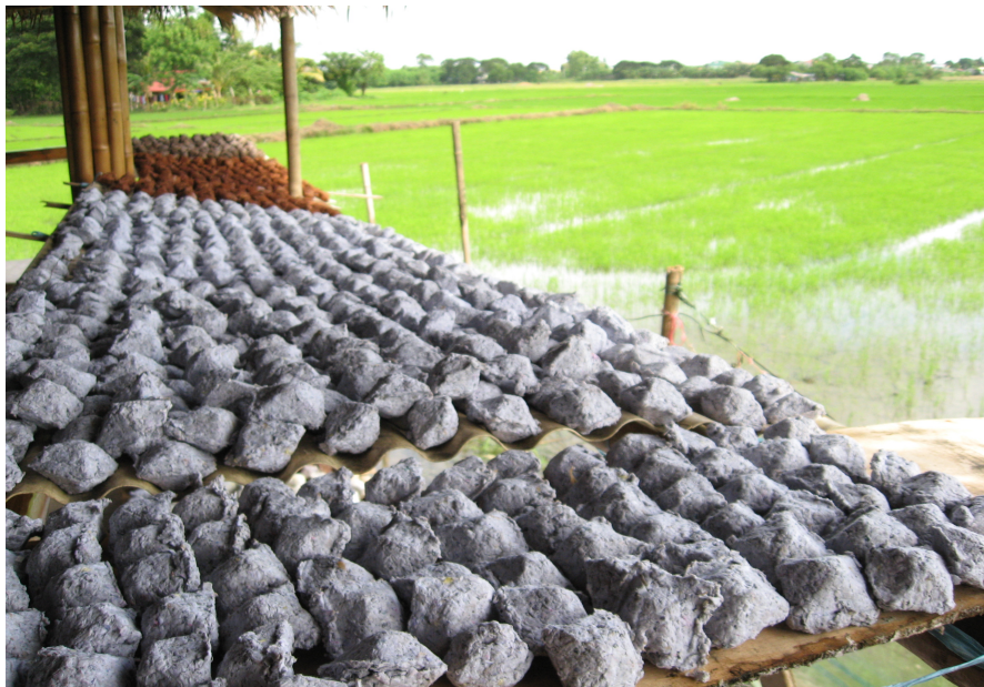
Figure 14. Pillow-shaped briquettes produced using the hand-press briquette molder
