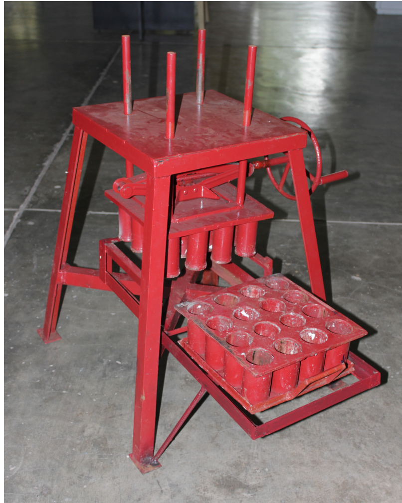
Figure 15. The first jack-driven briquetting machine developed for UCLA
