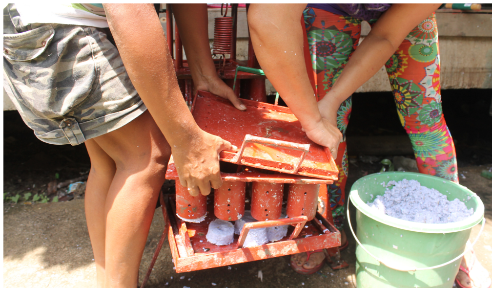
Figure 17. Removal of briquettes from the molder
