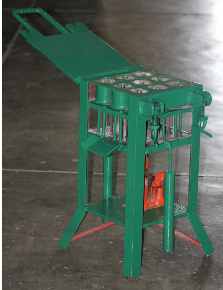
Figure 18. The second jack-driven briquetting machine developed for UCLA
