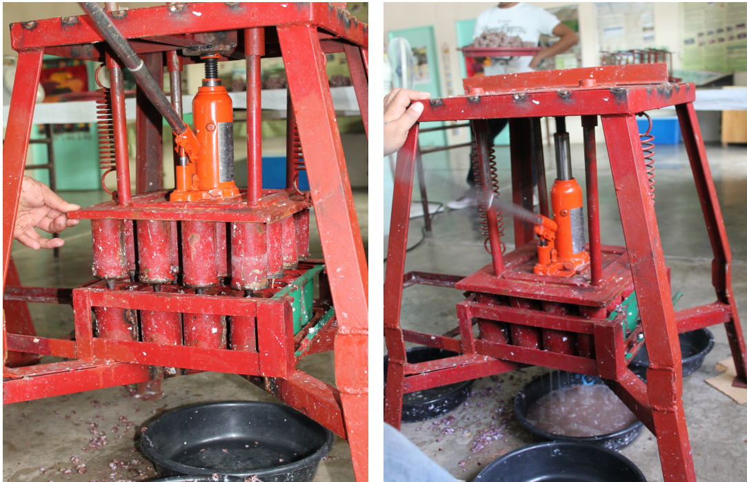
Figure 16. The hydraulic-type bottle-jack press briquetting machine in operation
