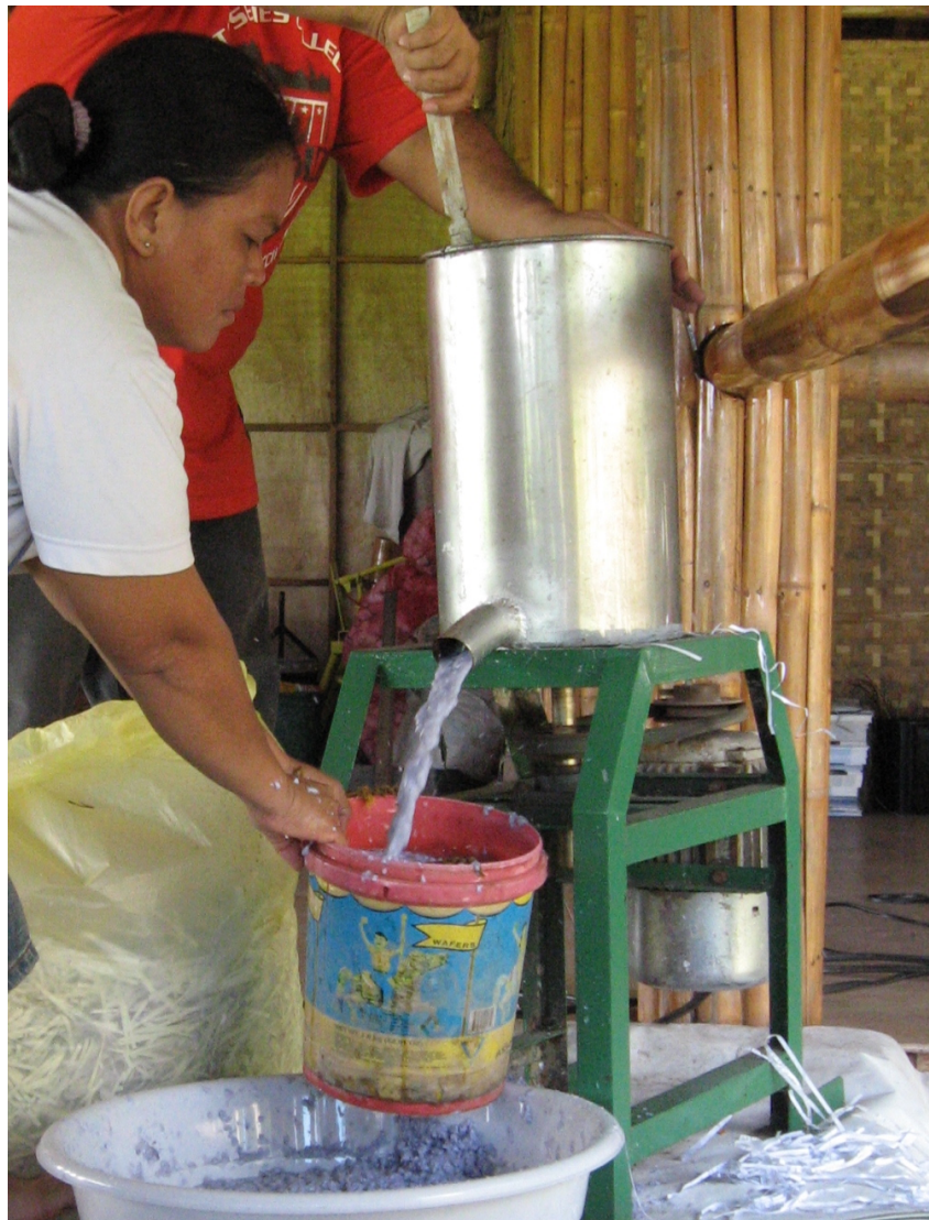
Figure 20. The pulping machine utilized during briquette production
