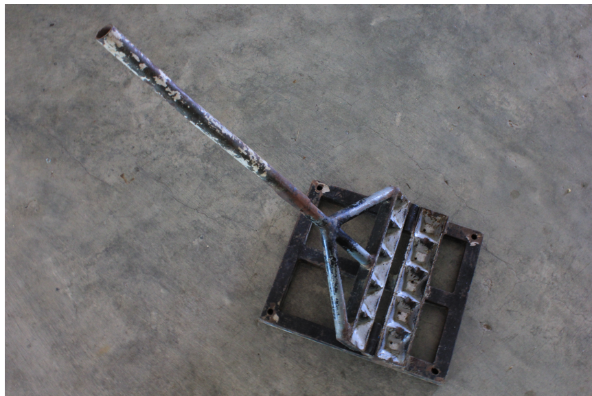
Figure 13. The second hand-press briquette molder with an extended handle
