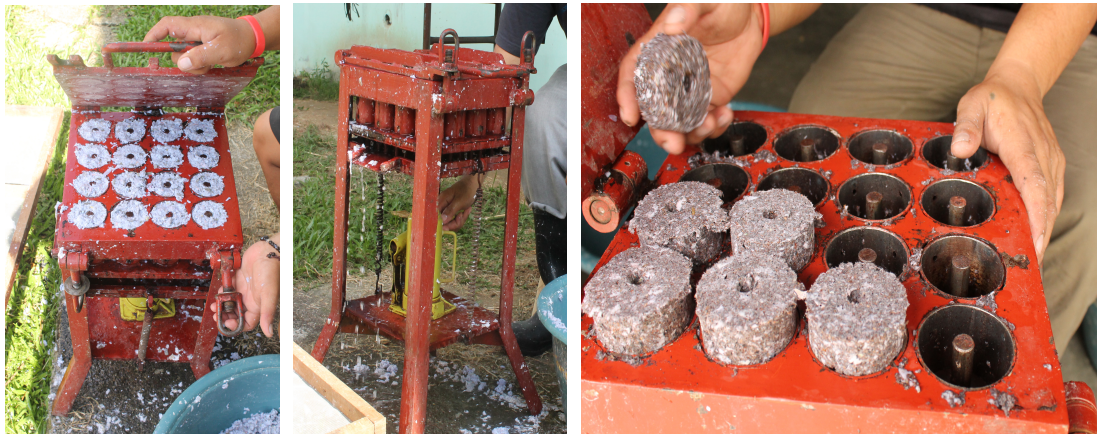
Figure 21. Briquetting of wastes showing the placement of mixtures in the molder, compaction of the materials and removal of briquettes produced from the molders
