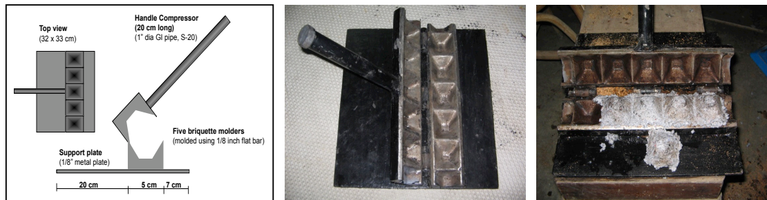
Figure 11. The first hand-press briquette molder developed with briquettes produced
