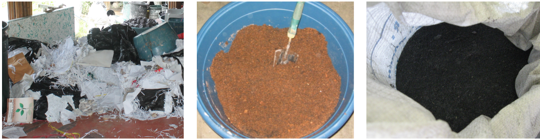
Figure 22. The materials used in briquette production, namely from left to right: waste paper, sawdust and carbonized rice husk
