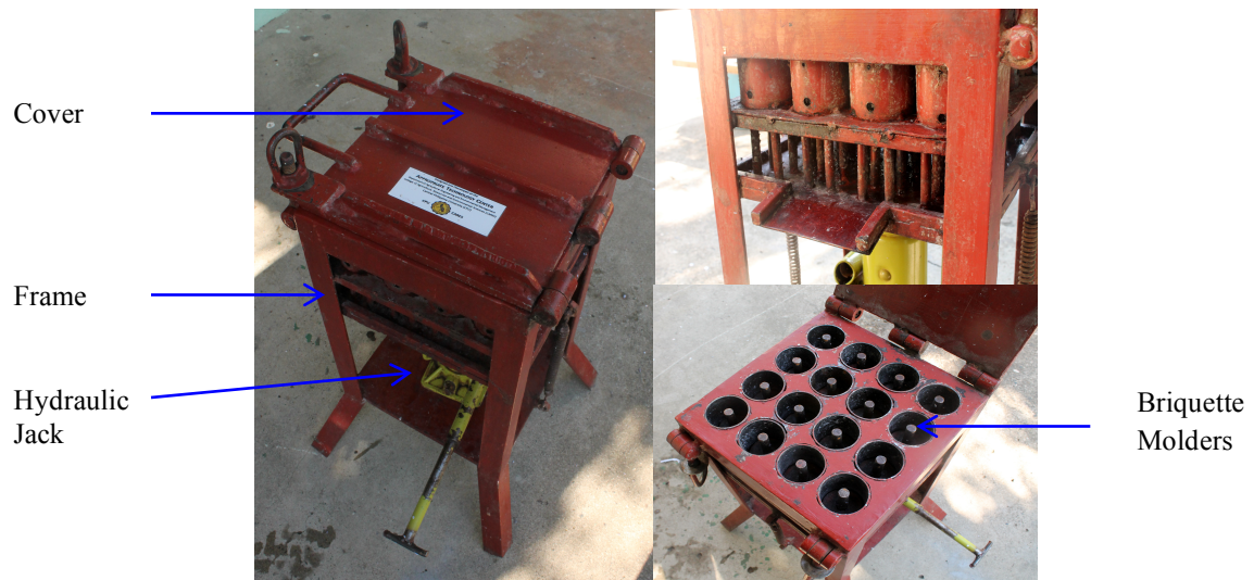
Figure 19. The final design of the hydraulic-jack driven briquetting machine to enhance briquette production
