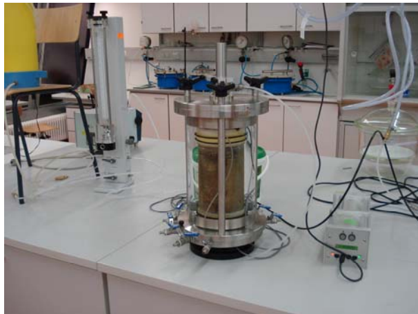
Figure 38. Calibration of triaxial cell with a steel dummy
