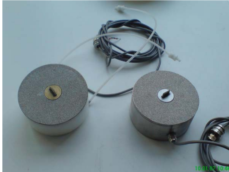
Figure 24. Bender elements installed in top cap and pedestal of a triaxial cell.
