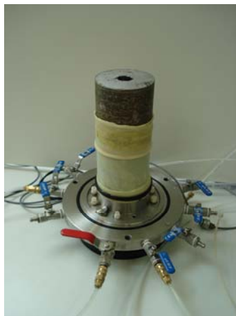
Figure 39. A steel dummy used to calibrate the triaxial cell
