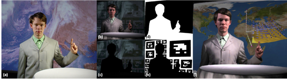
Figure 1: Real studio setting with physical back projection encoding adaptive imperceptible patterns (a), images captured by camera at 120Hz (b, c), computed foreground matte from real-time difference keying (d), extracted multi-resolution marker pattern for in-shot camera pose estimation (e), and composite frame with virtual background and 3D augmentation (f).
