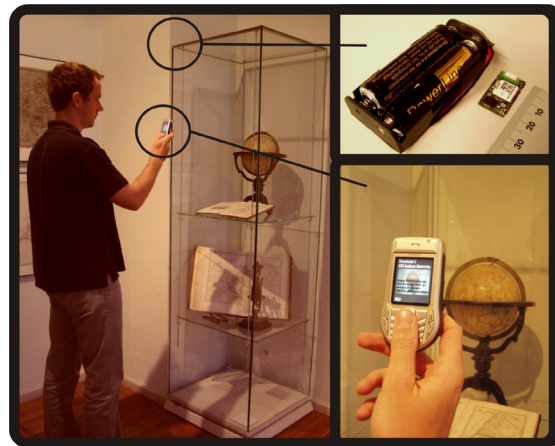
Figure 1: Mobile phone enabled guidance in a museum: On-device object recognition via computer vision combined with pervasive tracking through a coarse grid of Bluetooth emitters (emitter and battery pack shown above).
